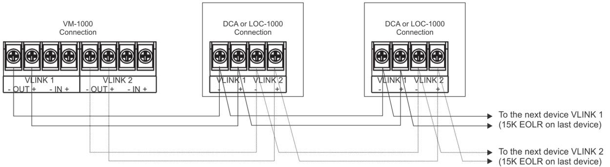
Figure 45. VM-1000 V-Link 1 and 2 Class B Wiring Example
