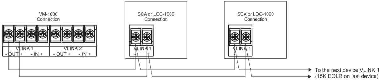
Figure 43. VM-1000 V-Link Class B Wiring Example
