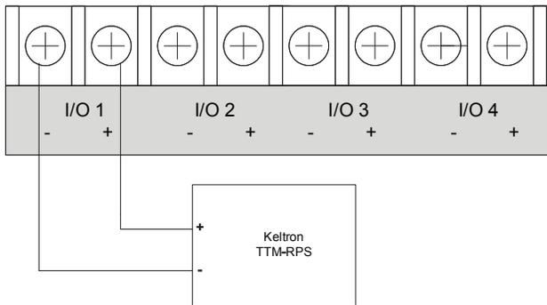
Note: IO circuit must be configured as a Reverse Polarity circuit
