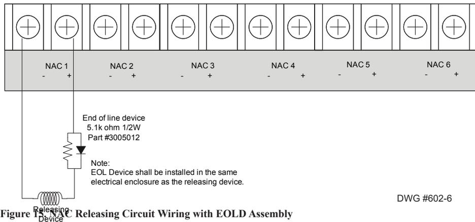
The maximum current is 3 amps. The maximum line impedance is calculated using the following formula.
