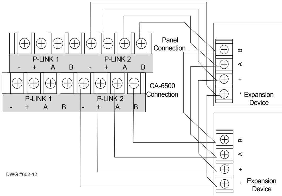
Figure 14. P-Link Class A Wiring Example Requires CA-6500
