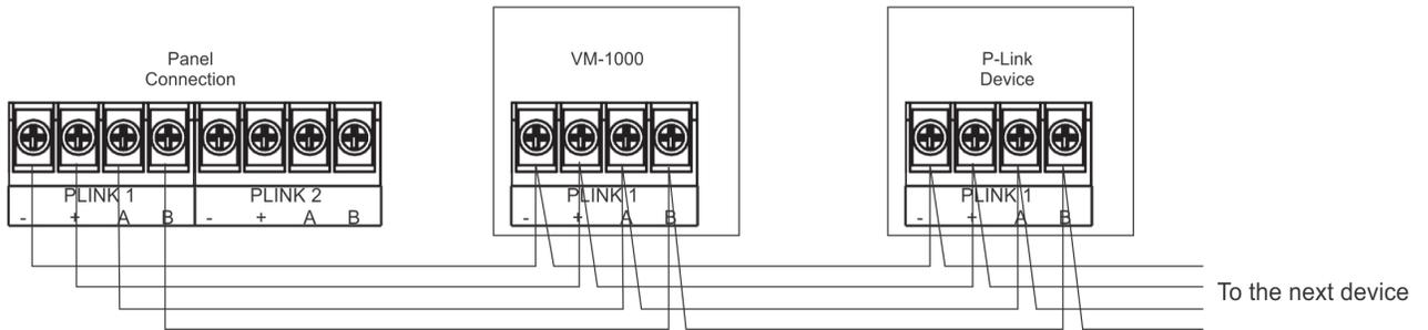
Figure 41. VM-1000 P-Link Class B Wiring Example
