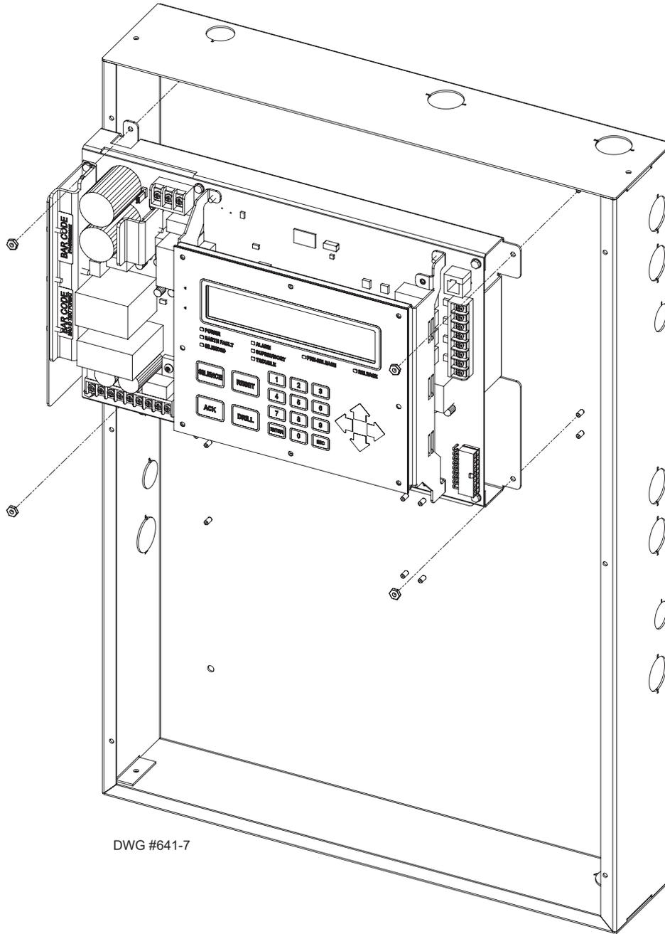
Figure 51. IPA-4000 Cabinet Showing Circuit Board Assembly
