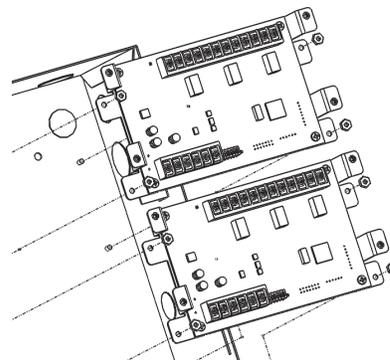
**Figure 34. IDC-6 Initiating Device Circuit Expander and IDC-6 Installation**
