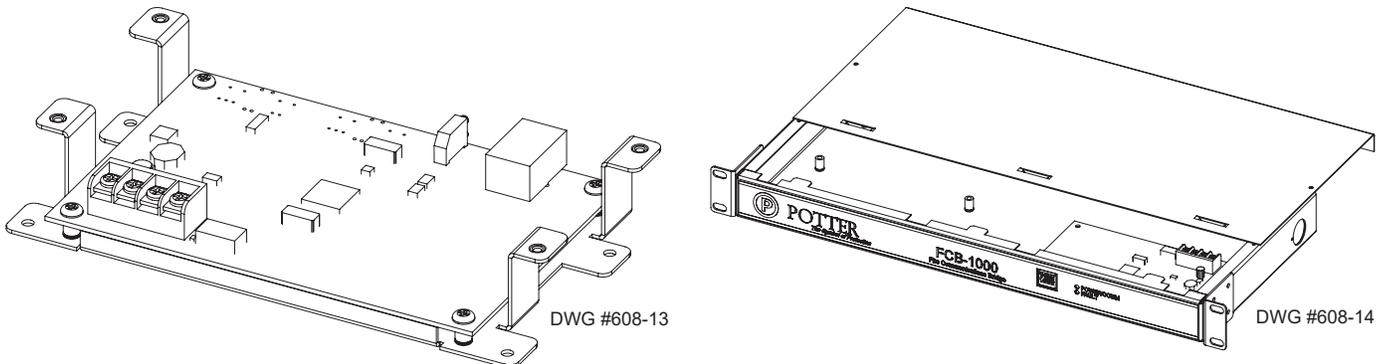
Figure 30. FCB-1000 Bridge & FCB-1000RM Showing Rack Mount
