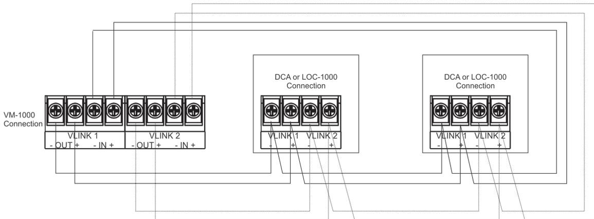
Figure 46. VM-1000 V-Link 1 and 2 Class A Wiring Example
