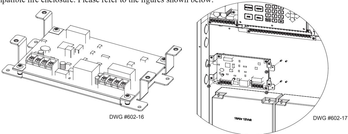
Figure 21. PAD100-SLCE / Nohmi Protocol SLCE-127 Board & Shown Installed in IPA-4000 Cabinet
