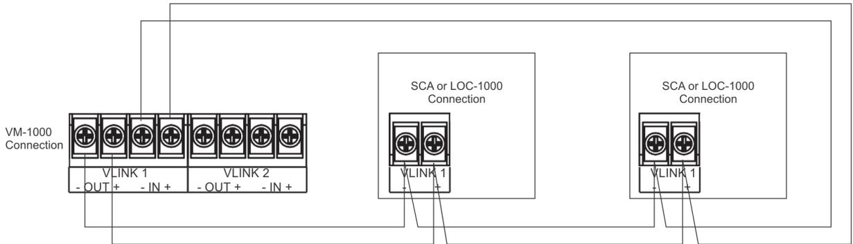
Figure 44. VM-1000 V-Link Class A Wiring Example
