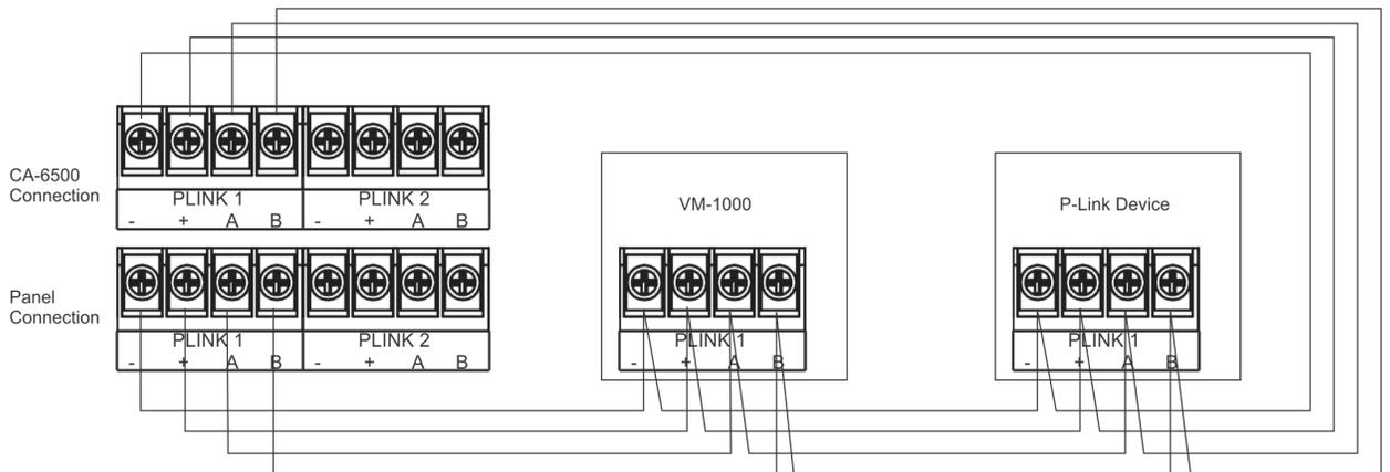
Figure 42. VM-1000 P-Link Class A Wiring Example
