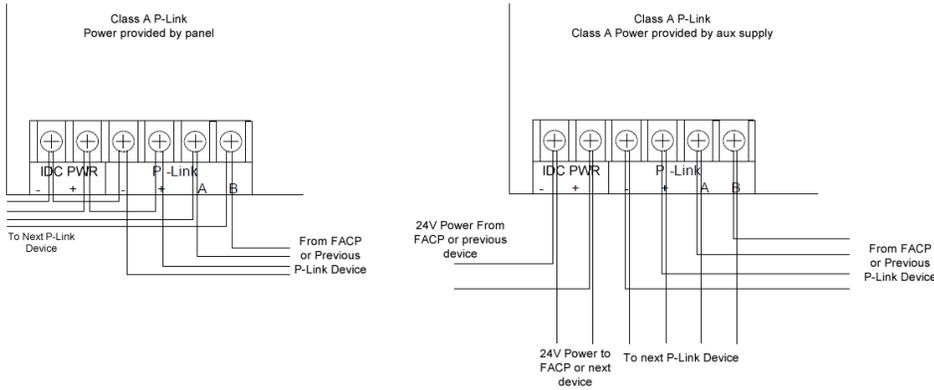
Figure 35. IDC-6 Class A Wiring
